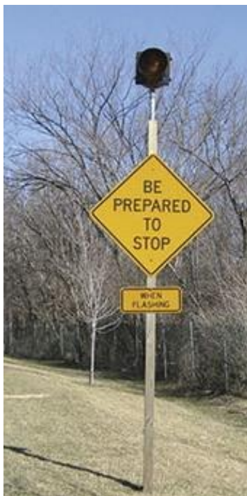
Advanced Warning Flasher (AWF)
